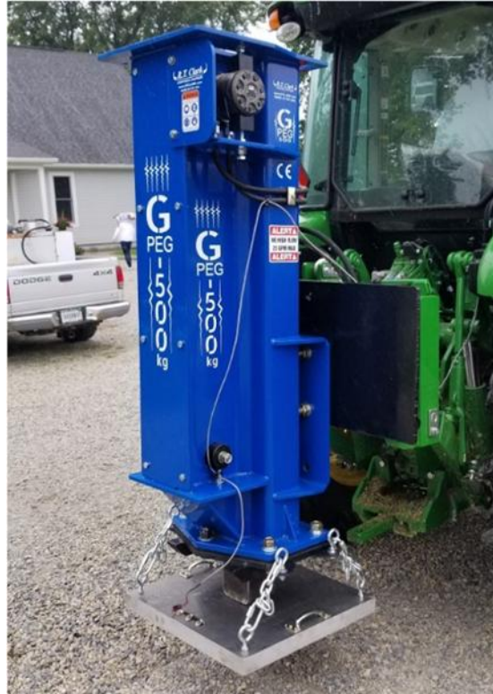
Figure 3-3: Weight Drop ('thumper') Unit Mounted to a Tractor
