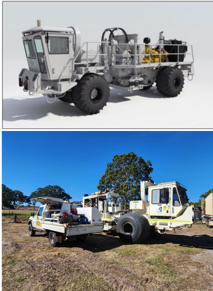
Figure 3-2: Vibroseis Trucks (Source: Sercel, 2020)
