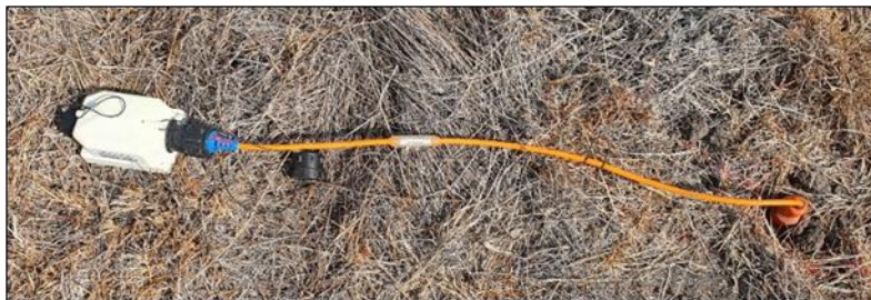
Figure 3-7: Wireless Geophone ('node') with Sensor Installed in Shallow Hole
