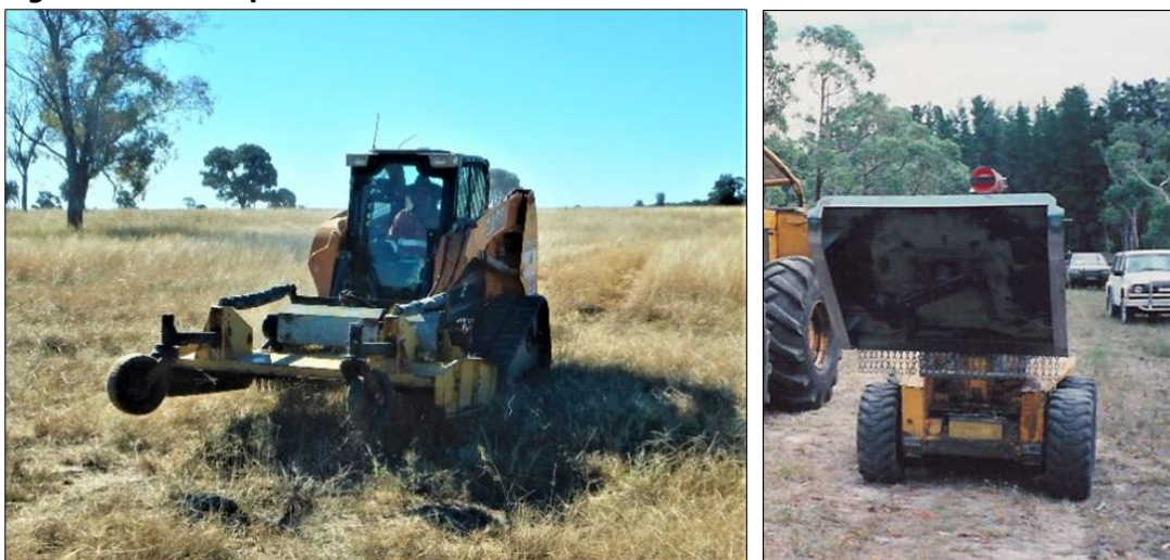
Figure 3-14: Bobcats with Vegetation Mulching Attachments (Source: Roberts, 2001)
